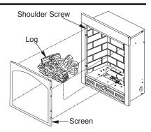
Figure 22 - Installing Log and Screen **OPERATING FIREPLACE**
